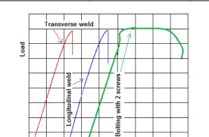
Table 3 Results of tensile strength and shear of the connections.
