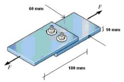
Figure 2 - Plates bolted to the shear test
