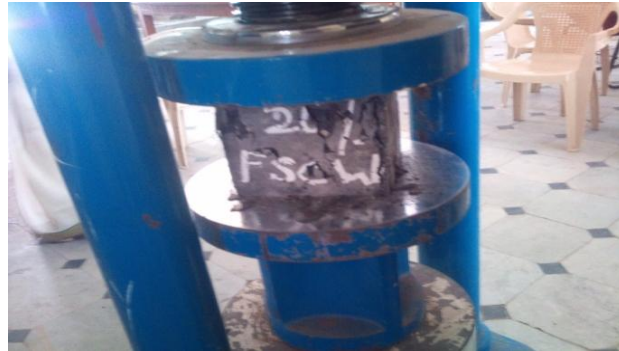
Fig. 9 Test Set - up for Cube Specimen
