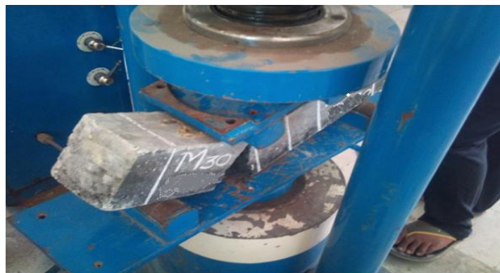
Fig. 13 Test Set - up for Prism Specimen
