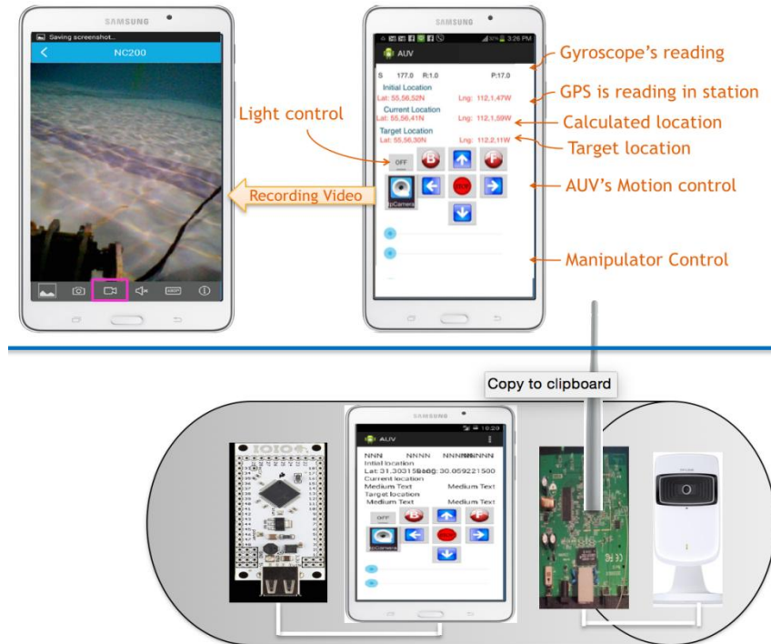
Fig. 4 Android application components and its view on server and enabling client to perform all commands while they are in the same LAN.
