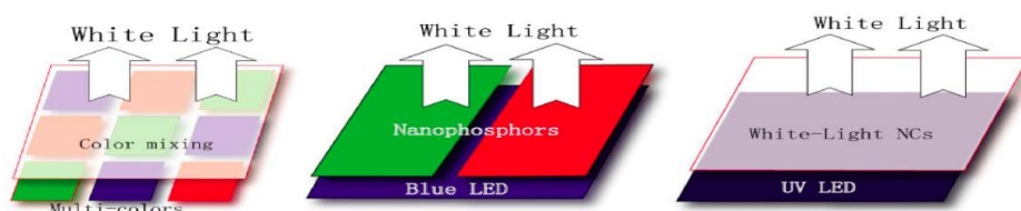
Figure 2 Schematic diagram of three methods obtaining white light Left) multi-color combination QLED; middle) light conversion QLED; right) Quantum dots and quantum well resonance energy transfer QLED
