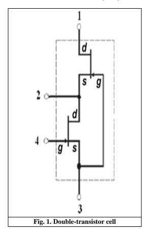
Creating a common contact to the source and gate regions of the primary transistor reduces the series resistance of the source and gate regions, excluding the input signal loss. This opens the possibility of its use as a stabilized current generator. Pinch-off voltage of the primary field-effect transistor is 0.8 V with a negative temperature coefficient and in additional field-effect transistor is 0.5 V - with a positive coefficient that provides a thermally stable mode, fig. 2.
