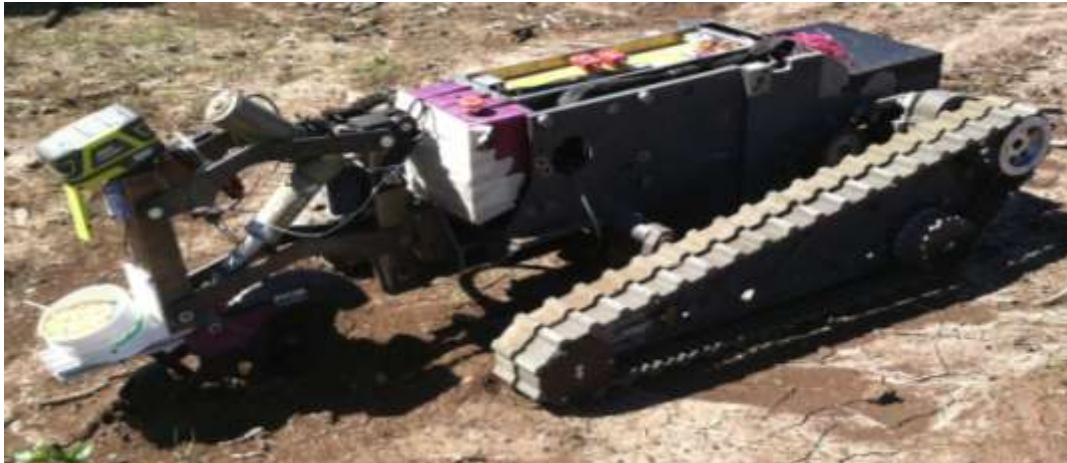
Figure 1: KSU- BAE UGV with a prototype planter sowing wheat seed.
