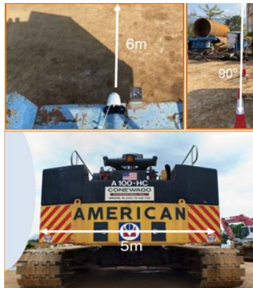
Fig 5: Connecting cameras to the machinery
