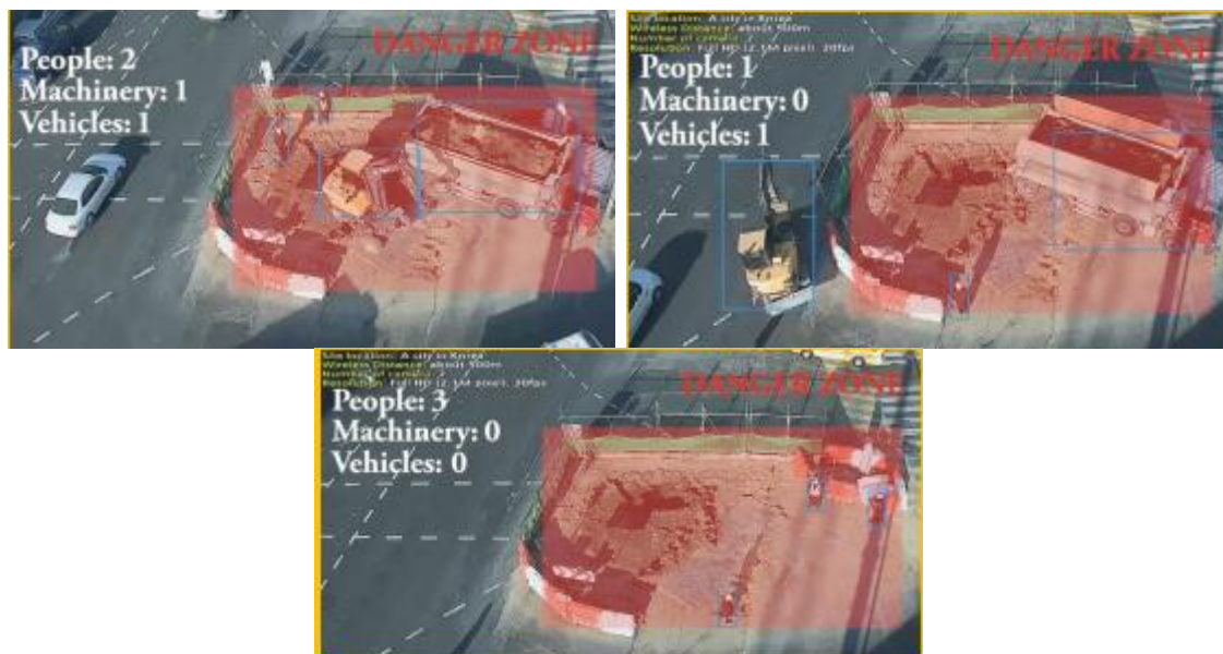
Fig 7: Audio-visual alerts on machine collision instances
