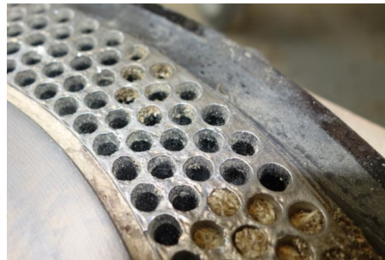
Fig. 7 Uniform abrasive wear of flat die surface
