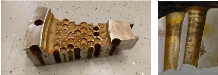
Fig. 13 Damage to the pressing channels of the die by pitting
