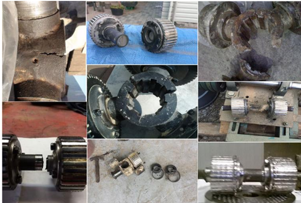
Fig. 16 Different types of wear and damage to the pressing rolls [23]
