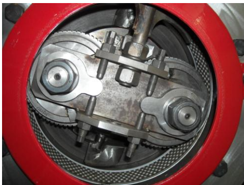
Fig. 4 Pressing rolls arrangement of ring die pelleting press
