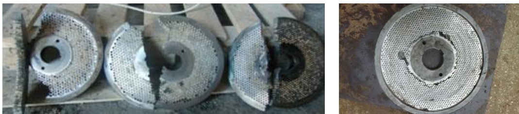
Fig. 14 Damage to the flat die by fatigue fracture [23]
