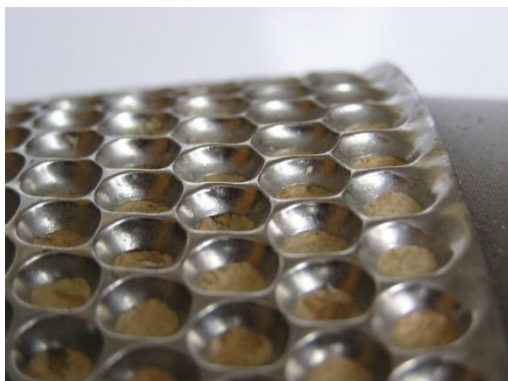
Fig. 8 Detail of the wear of the perforated surface of the pressing rolls
