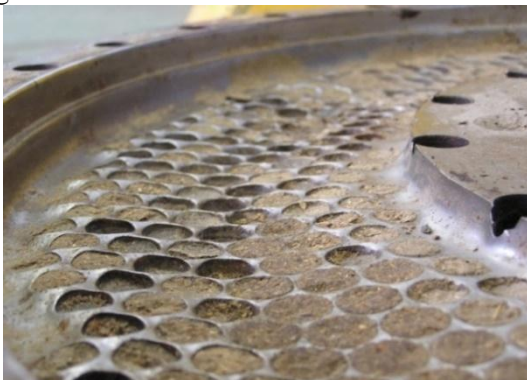
Fig. 6 Deep wear of the die surface
