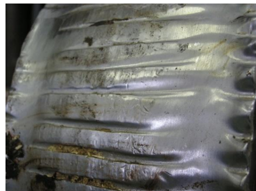
Fig. 9 Detail of deep wear of the grooved working surface of the roll
