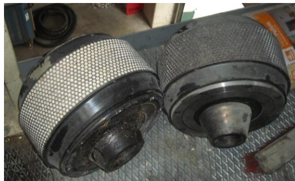
Fig. 5 Construction of pressing rolls of the ring die pelleting press
