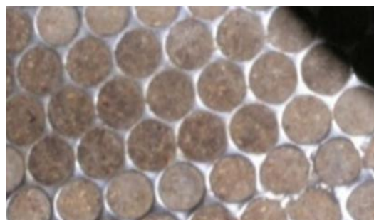
Fig. 12 Wear of the die surface by "honeycombing"
