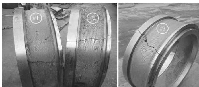
Fig. 15 Damage to the ring die by fatigue fracture [14]
