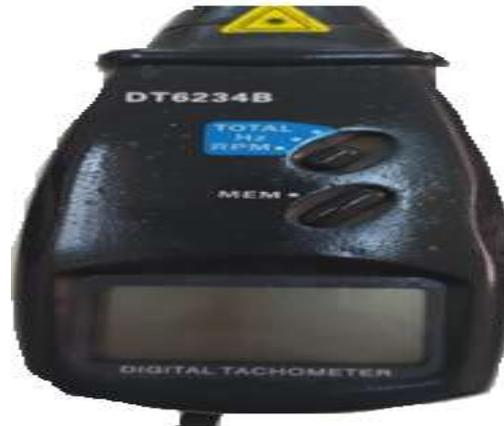
**Fig. 5 Digital tachometer DT6234B**
