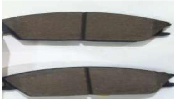
**Fig. 3 Disc brake pad of test rig**
