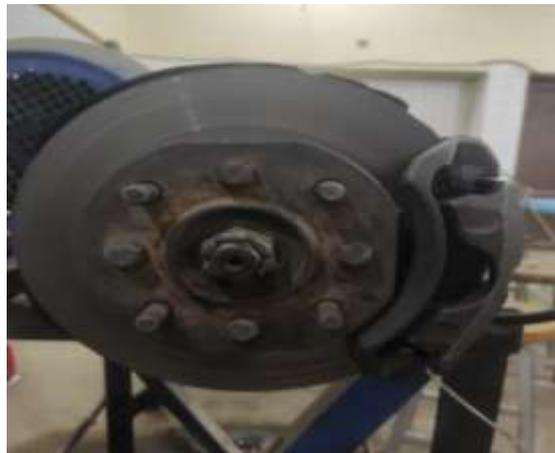
Fig. 2 Disc brake system of hyundai excel 2005 model
