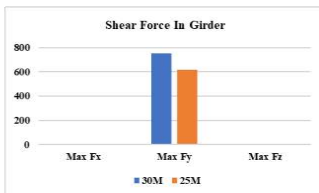
Figure. 5 Shear force on Different Span
