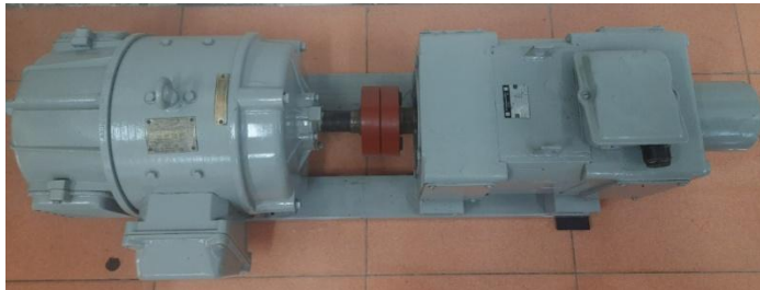
Fig 2. 1. The experimental setup consists of a dc motor, a generator, and a tachogenerator.
