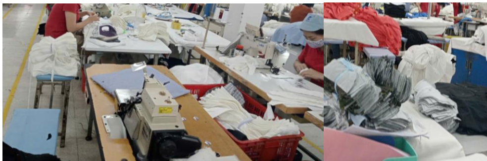
Figure 3.1. Wastes related to machine downtime, work-in-process (WIP) inventory, and overproduction [7]
