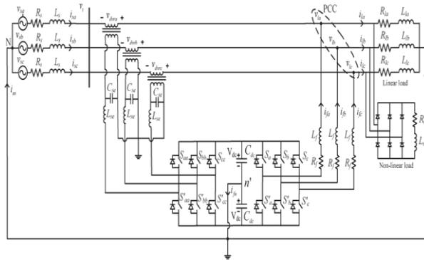
**Fig.2:** Power circuit of neutral-clamped VSI topology-based UPQC
