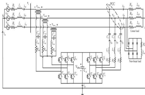
**Fig.3:** Equivalent circuit of proposed VSI topology for UPQC compensated system
