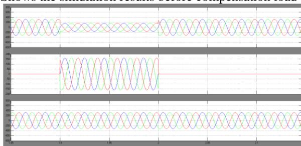
**Fig. 9:** Shows the Terminal voltages with sag, DVR-injected voltages and load voltages after compensation
