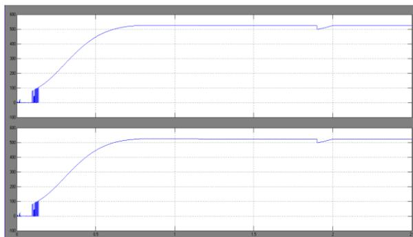
**Fig. 6:** Shows the DC and fundamental values of voltage across series capacitor and inverter output voltage
