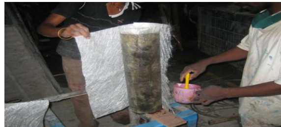
Fig.2 Wrapping under Progress
