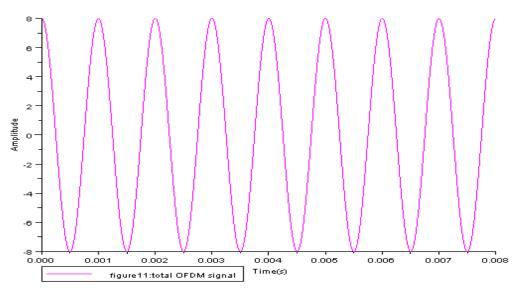
From the figure 1 to 4, we have respectively the OFDM signals at the first chip time, at the second chip time, at the third chip time and at the fourth chip time. The figure 5 represents the OFDM signal for the first bits of the symbols  $A_0$ ,  $A_1$ ,  $A_2$ ,  $A_3$ . Thus it represents the sum of the OFDM signals obtained from the first chip time to the fourth chip time.
