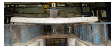
(h) Slab S6; HSCC with steel fibers (1.5%)
