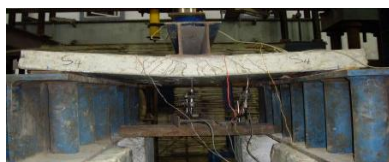
(g) Slab S4; HSCC with steel fibers (0.75%)
