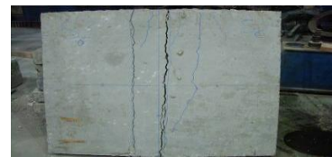
(f) Slab S6; HSCC with steel fibers (1.5%)
