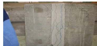
(b) Slab S2; SCC without steel fibers
