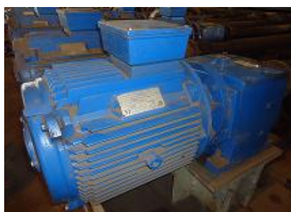
Fig. 2. Unregulated motor self cooling arrangement
