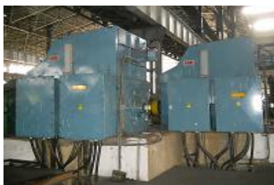
Fig. 6. Regulated AC squirrel cage motor with external cooling arrangement.
