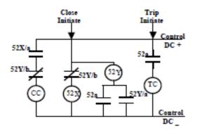
The CBM IED monitors 15 electrical signals from the circuit breaker control circuit shown in Figure 1. The signals are generated during either tripping or closing of the breaker. Of these 15 signals, 11 are analog and 4 are status signals.
