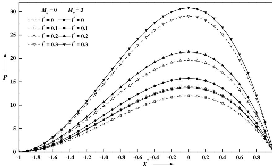
Figure 2. Variation of nondimensional Pressure  $P$  with  $x^*$  for different values of  $M_0$  and  $l^*$  with  $h^* = 0.4, y^* = 0$ .
