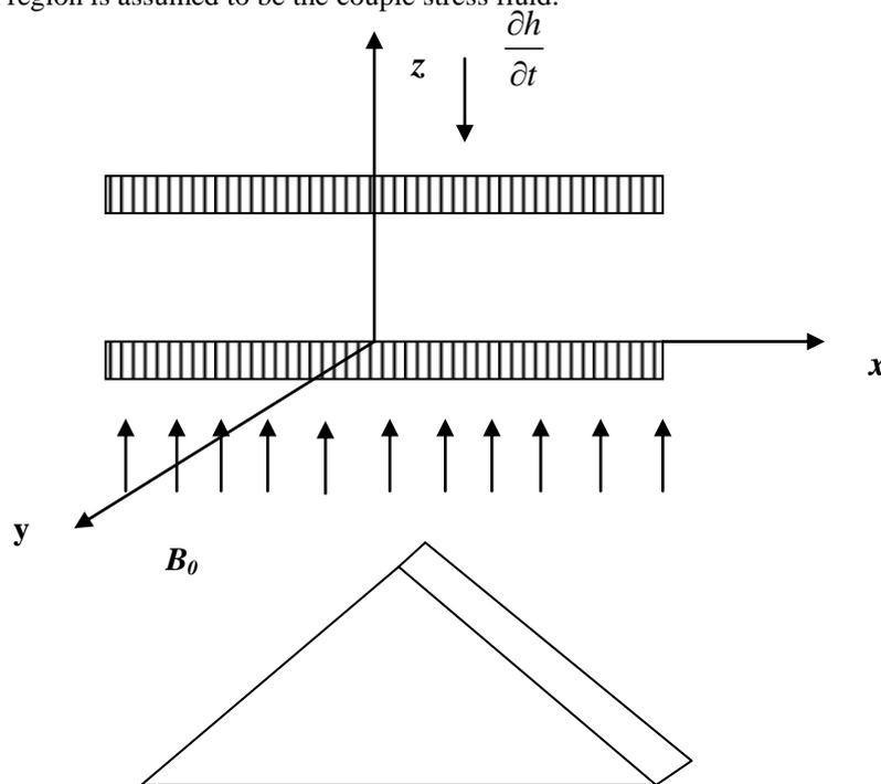
Fig. 1 Schematic diagram of the Rectangular Bearing
