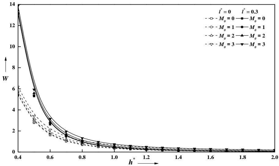
Figure 5. Variation of nondimensional Load carrying capacity  $W$  with  $h^*$  for different values of  $l^*$  and  $M_0$ .
