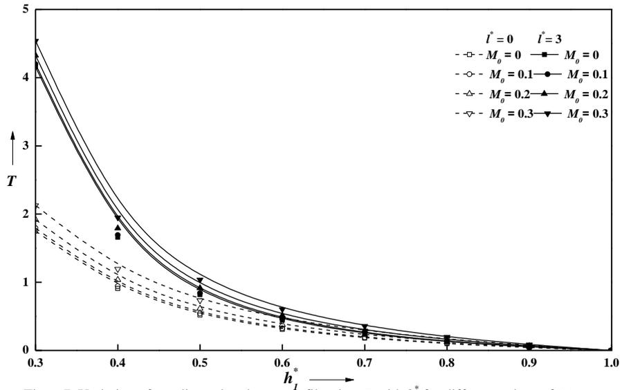
Figure7. Variation of nondimensional squeeze film time  $T$  with  $h_1^*$  for different values of  $M_0$  and  $l^*$ .
