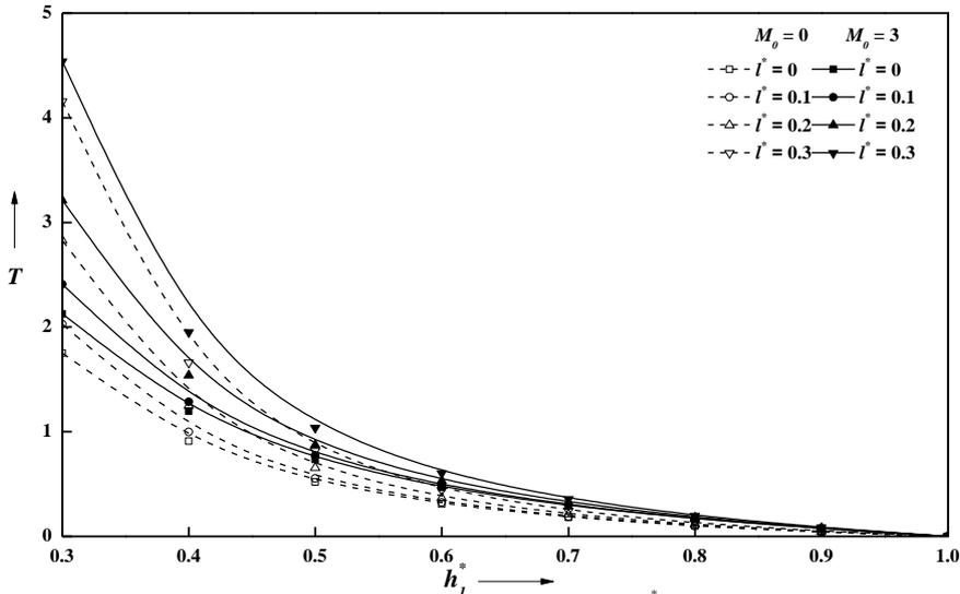
Figure 6. Variation of nondimensional squeeze film time  $T$  with  $h_1^*$  for different values of  $M_0$  and  $l^*$ .
