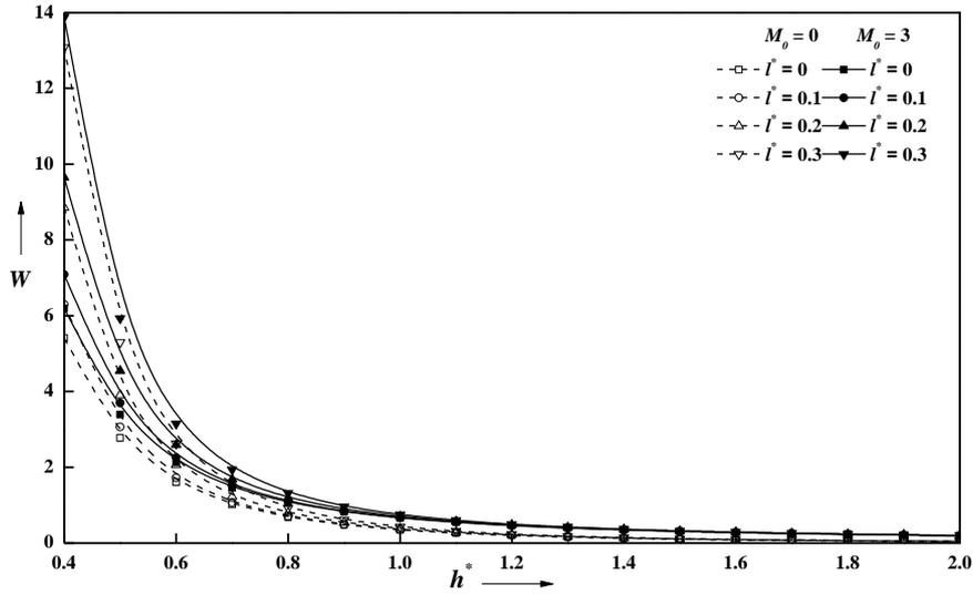
Figure 4. Variation of nondimensional Load carrying capacity  $W$  with  $h^*$  for different values of  $M_0$  and  $l^*$ .
