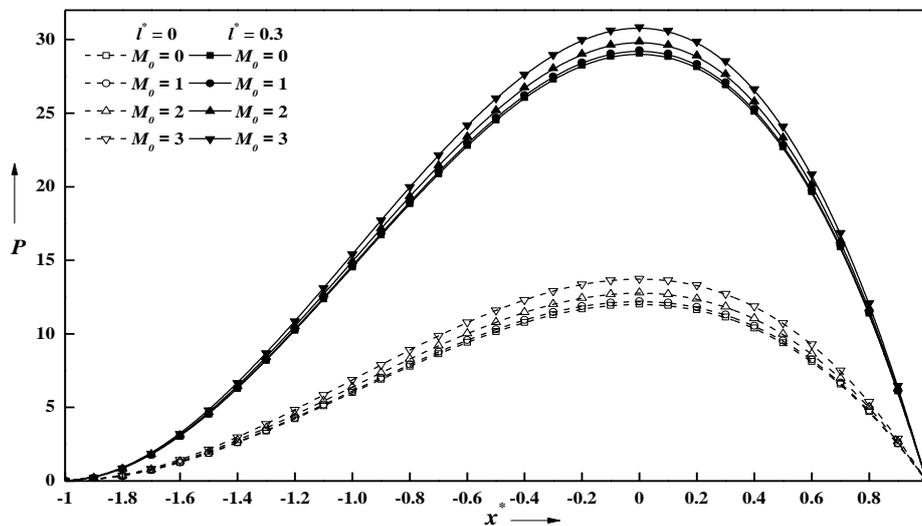
Figure3. Variation of nondimensional Pressure  $P$  with  $x^*$  for different values of  $M_0$  and  $l^*$  with  $h^* = 0.4, y^* = 0$ .
