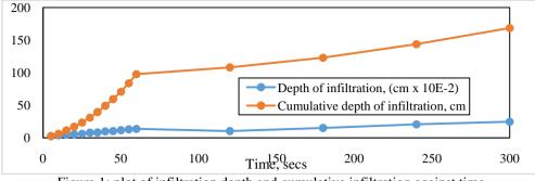
Figure 1: plot of infiltration depth and cumulative infiltration against time
