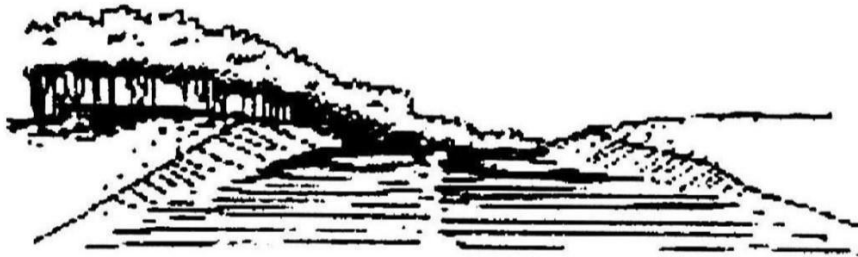
Tree planting used to provide indication of alignment beyond crest
