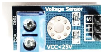
Fig.2 Voltage Detection Sensor Module
