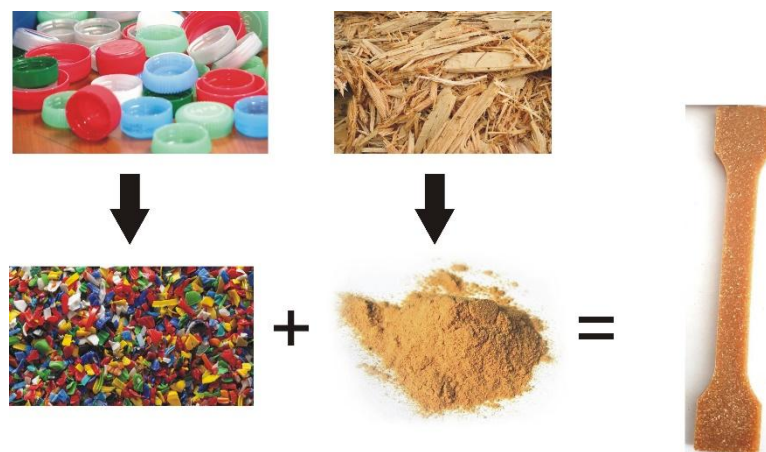
Fig. 2 Schematic view of raw material treatment and samples production
