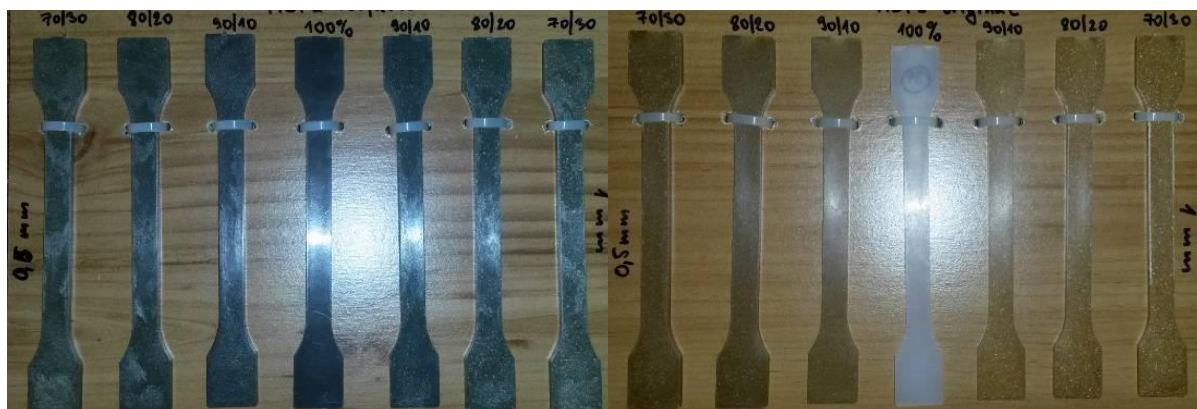
Fig. 3A WPC samples based on recycled HDPE (left) and a WPC sample based on virgin HDPE (right)
