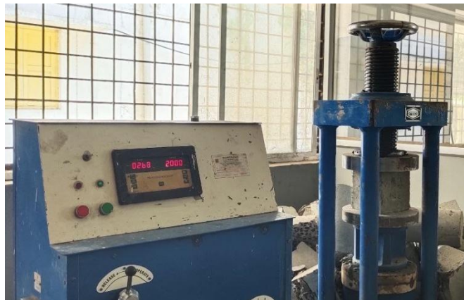
Figure 1: Compressive Strength Test
