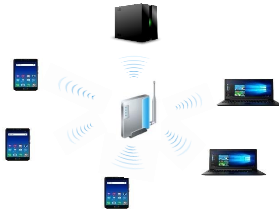
Figure 3. Physical Network Topology of the System
