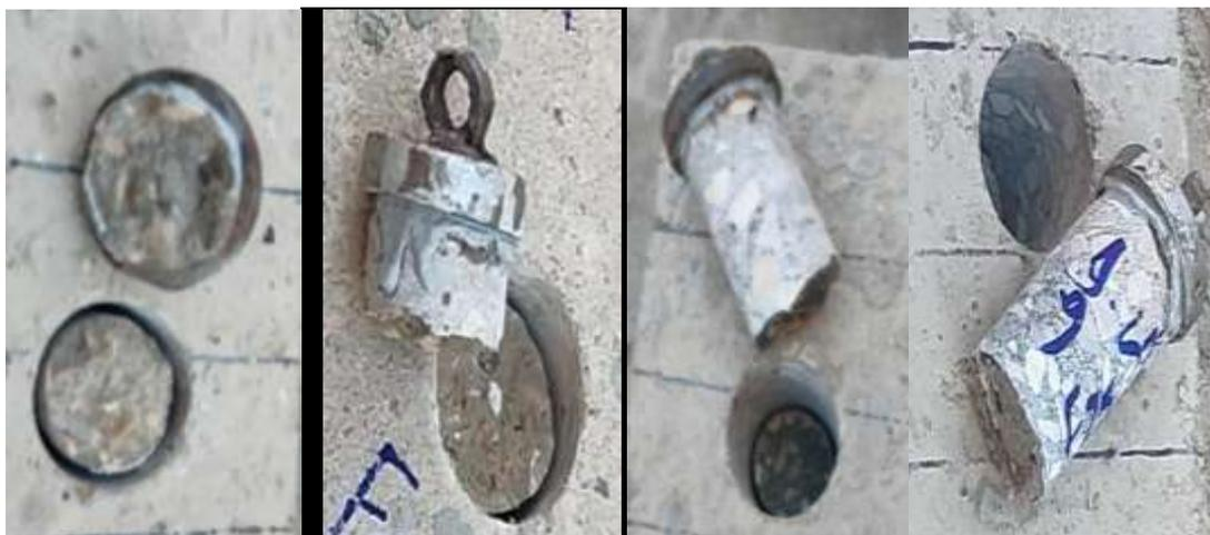
Fig. 8: Failure of the pull-off specimens in a) top surface of repair material, b and c) repair material, d) substrate concrete
