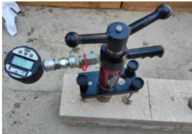
**Fig. 3: Pull-off test setup**
