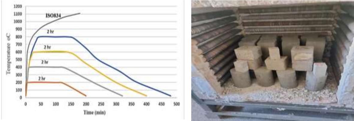
**Fig.6: a) Fire curves, b) Concrete specimens in electrical furnace**
