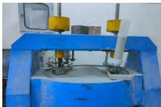
**Fig. 4: Abrasion resistance test machine**
