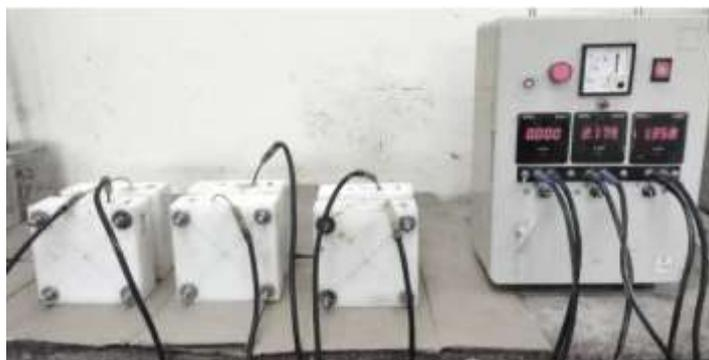
**Fig. 5. Rapid chloride penetration test setup**
