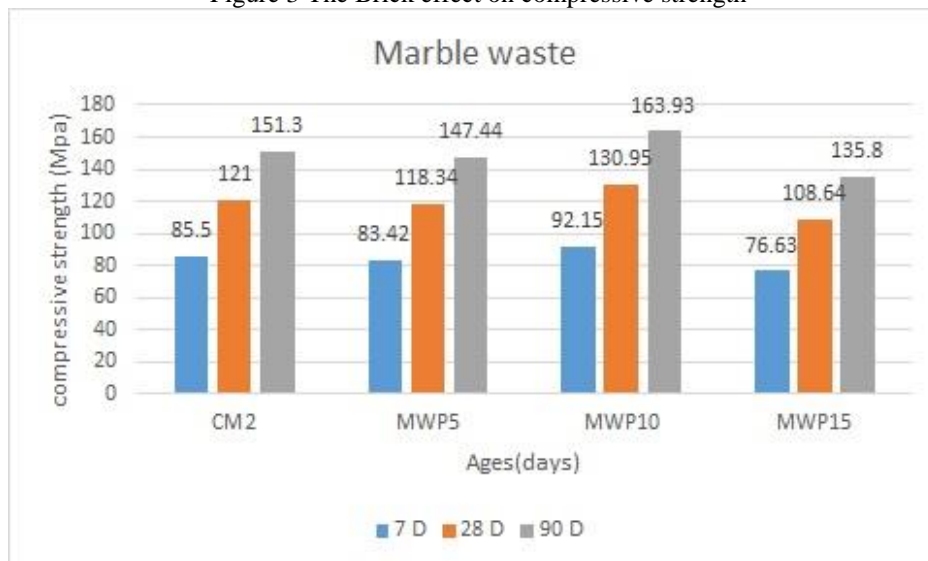
Figure 4 The Marble effect on compressive strength
