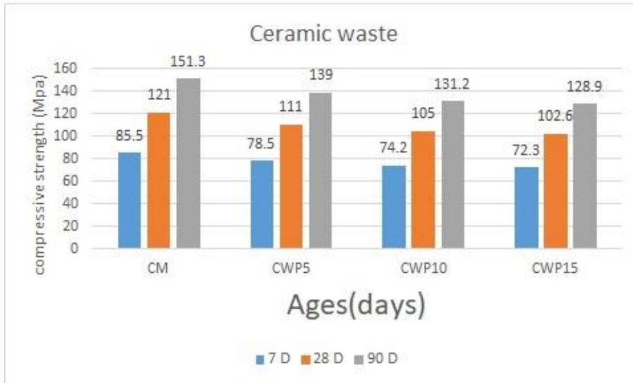
Figure 2 The ceramic effect on compressive strength
