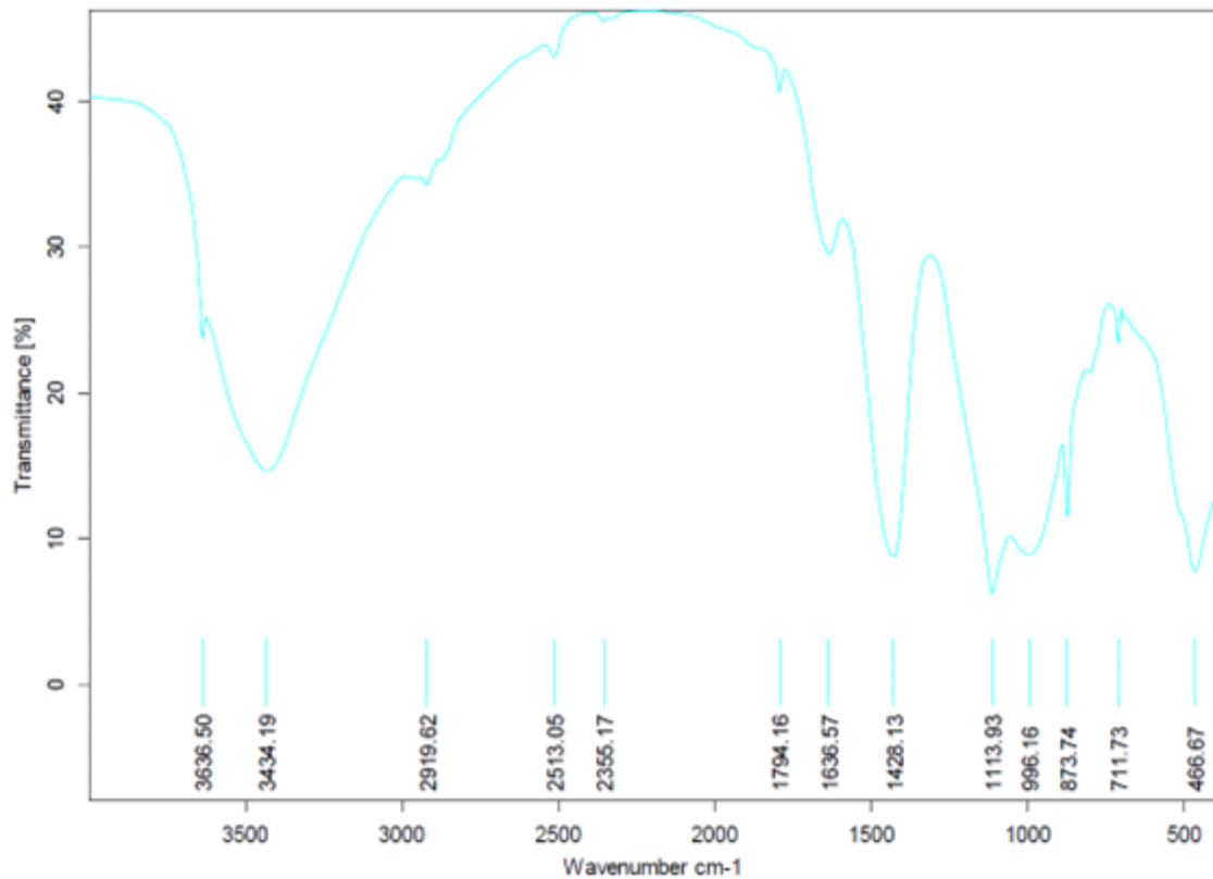
Figure. 25 FT-IR results of UHPC (MWP)
