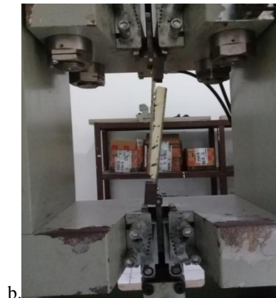
b. Sample were tested under tension shear load
