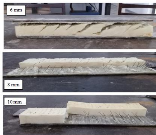
Figure 5 photos of specimen failure after shear test
