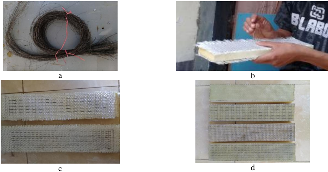
Figure 1 a. sugar palm fiber b. hand running stitch on PUR-fiberglass c. PUR-fiberglass has been sutured d. sandwich composite has been completed
