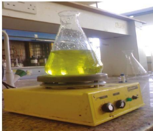
Fig.1. shows solving of catalyst mixture in oil (60°C)
