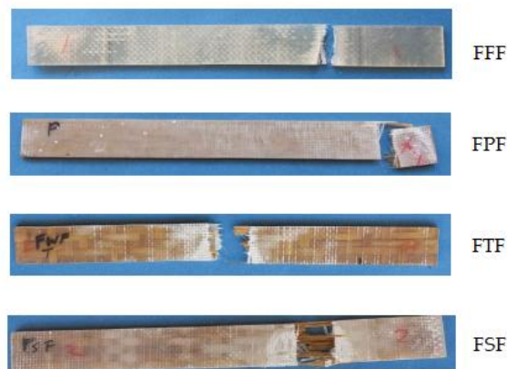
Figure 6 Composite tensile fracture
