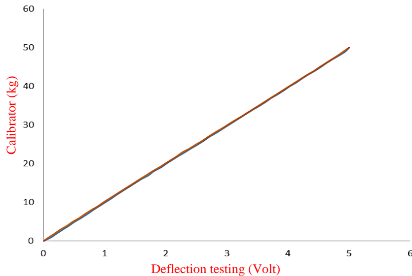
Fig. 10. Hysteresis graph for deflection measuring instruments
