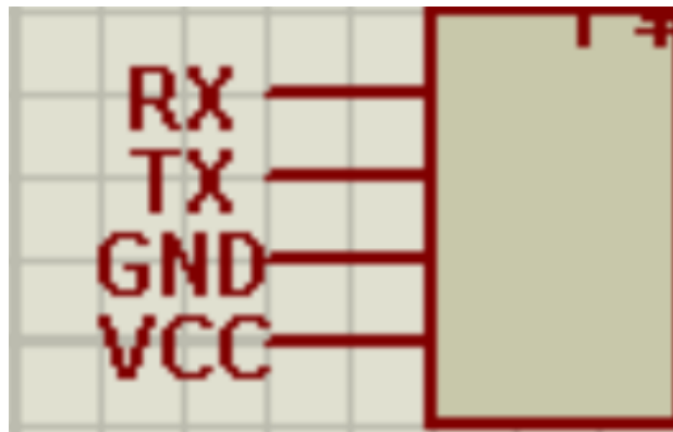
Figure 3.15 ESP8266Wi Fi Module Circuit Connection Diagram
