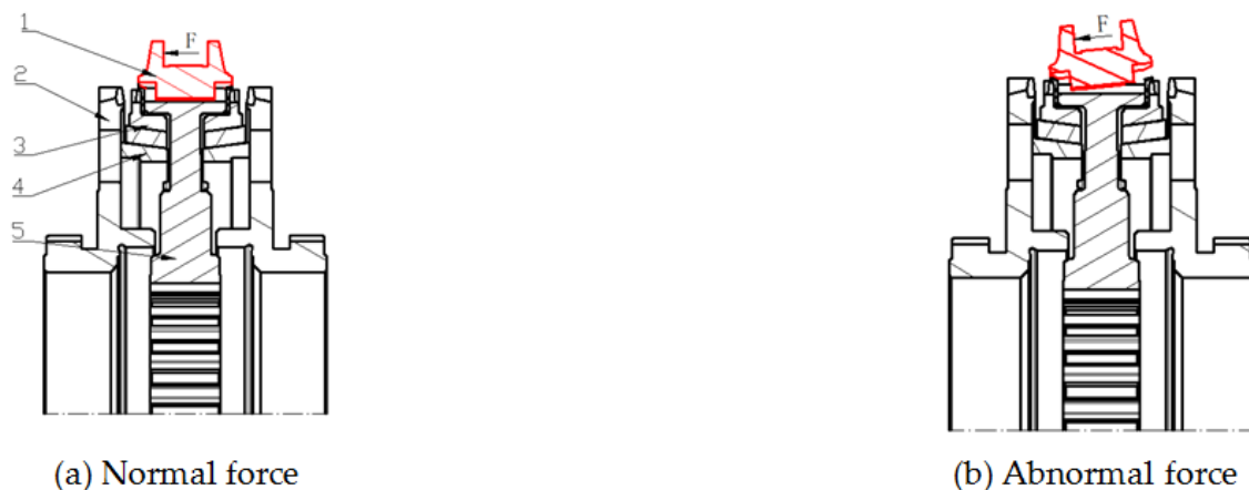
1-Jointing set, 2- Jointing gear ring, 3- Composite synchronous ring outer ring, 4- Composite synchronous ring inner ring, 5- Spline Hub
