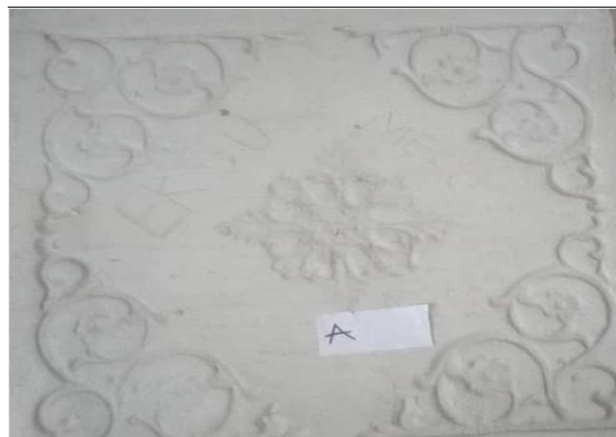
Plate 1: Sample of Ceiling board with a unique design after drying
