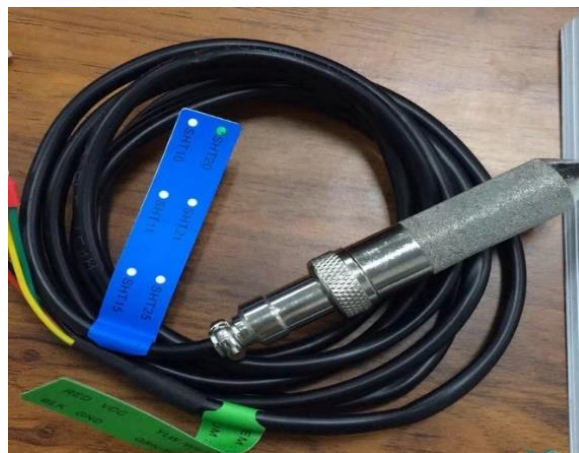
Figure 3-4 Soil temperature and humidity sensor
