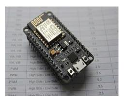
ATmega328 is commonly used in many projects and autonomous systemswhere a simple, low-powered, low-cost micro-controller is needed Node MCU is an open source IoT stage. It incorporates firmware which keeps running on the ESP8266 Wi-Fi Scow from Expressive Systems, and equipment which depends on the ESP-12 module.
