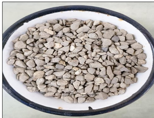
Figure 1(c) Gravel Particles passing 10.0 mm IS Sieve and retained on 4.75 mm IS Sieve
