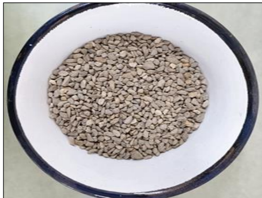
Figure 1(b)-Sand Particles passing 4.75 mm IS Sieve and retained on 2.0 mm IS Sieve
