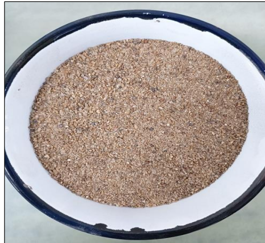
Figure 1(a)- Sand Particles passing 2.0 mm IS Sieve
