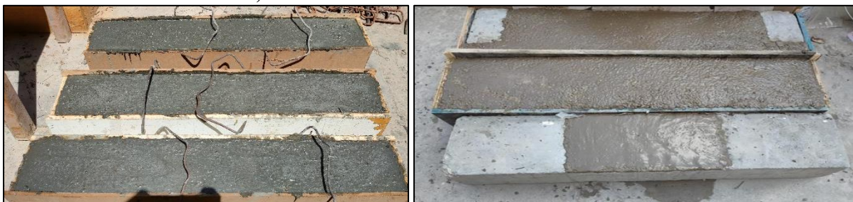
b) Concrete beams after casting
