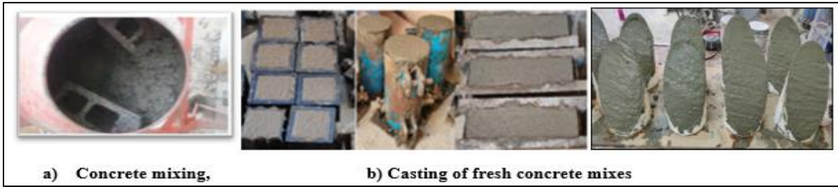
Fig. 1: Mixing and casting of concrete mixes
