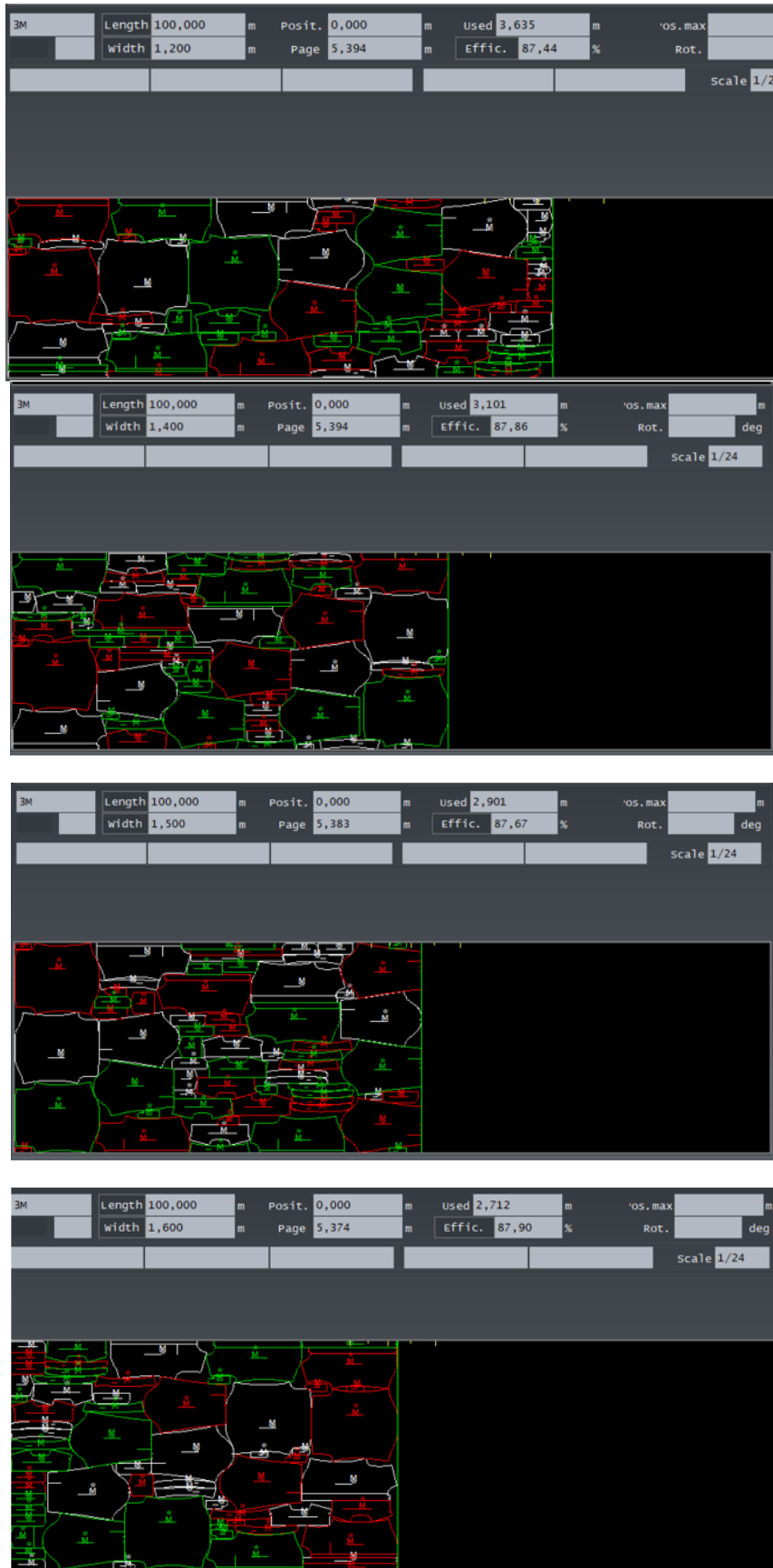
Figure 1. Size M shirt marker with different fabric widths
