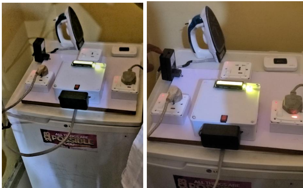
Figure 8 (a): Relay turns off after sensor detects absence. Figure 8 (b): Relay turns on switch after sensor detects presence
