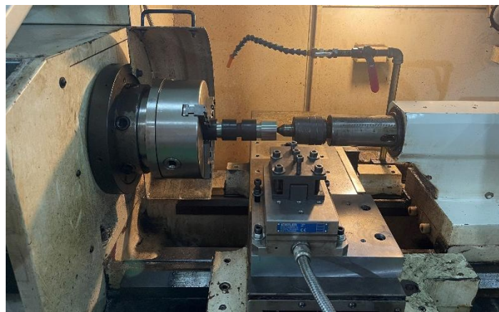
Figure 1. Device set-up of hard turning experiments
