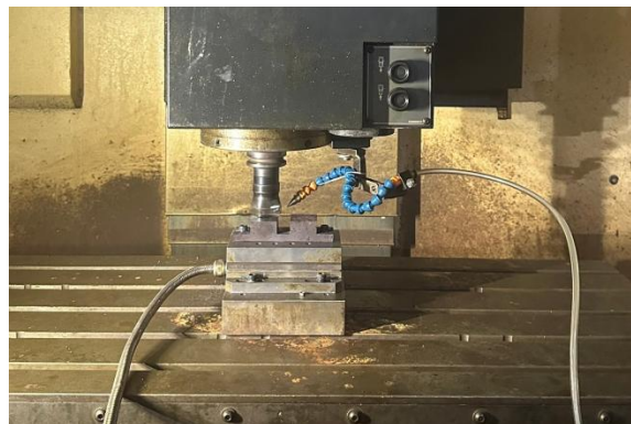
Figure 1. Device set up for hard milling experiments
