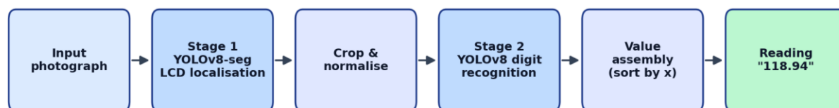
Figure 1. Overview of the proposed two-stage caliper-reading pipeline.
