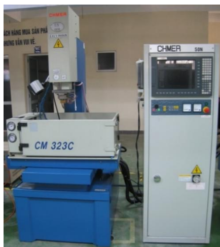
Figure 1. CM 323C electrical discharge machine
