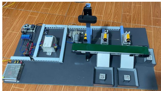
Fig. 2 Product classification model based on color and shape using the OpenCV library [3], [9].
