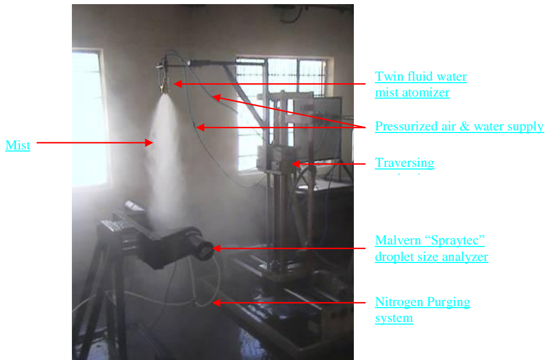
Figure 3: Atomizer characterization facility
